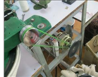
Photo of non-conformity NC-The factory did not install belt protective safeguard for the seaming machine.JPG
