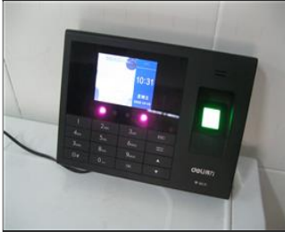
Photo of the inside of the main production hall Face recognition and fingerprint scanning attendance machine.JPG
